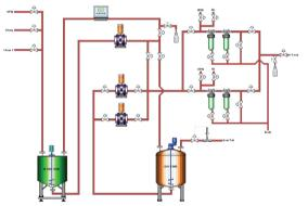
Configuration showing one blend tank, one day tank, redundant dispense pump, dispense filtration, and stirrer devices
